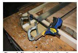
Figure 9 Clamp the boards to the rails as shown.
