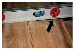
Figure 2 Board is humped indicated by space between board and level on right
