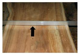
Figure3 Board is cupped on both sides.
