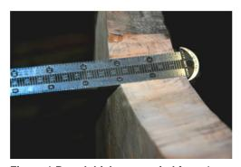
Figure 1 Board thickness varied from 1 1/2" to 2"
