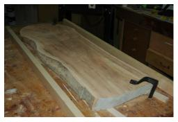
Figure 4 Cut base rails and place parallel near board
