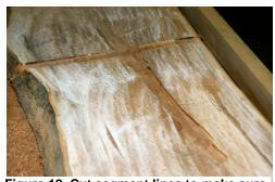
Figure 12 Cut segment lines to make sure that the router bit has not slipped
